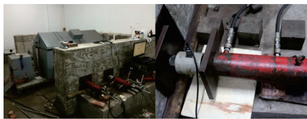
(a) 实验整体布置 (b) 千斤顶及压力传感器 (a) Experimental layout (b) Jack and pressure sensor
