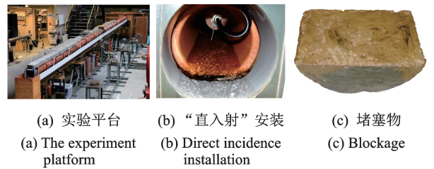
Fig.1 Blockage detection system based on acoustic technology
