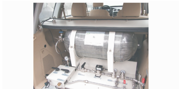
图 3 车用纤维缠绕储氢容器工作示意 Fig.3 Hydrogen on-board storage tank under fatigue loading
