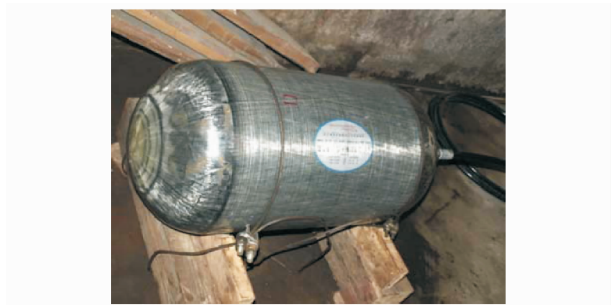
图 2 疲劳加载中的储氢容器 Fig.2 Hydrogen on-board storage tank under working condition
