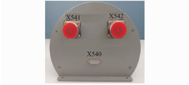
图 10 中北大学研制的 NUC-SD02 数据存储器 Fig. 10 NUC-SD02 data storage device developed by North University of China
