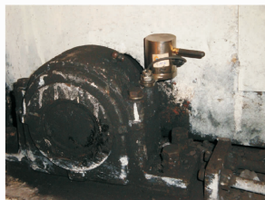
(b) 安装在滚筒轴承座上 (b) Installation position for roller bearing seat
