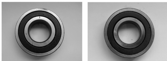
(a) 内圈故障 (a) Inner race defect (b) 外圈故障 (b) Outer race defect
