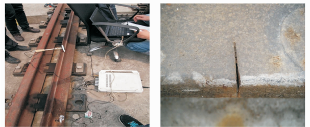
(a) 实验环境 (b) 裂纹伤损 (a) Experimentale environmen (b) Turnout flaw
