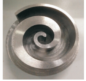
图3 待测变截面涡旋盘 Fig. 3 The non-uniform scroll part to be measured
