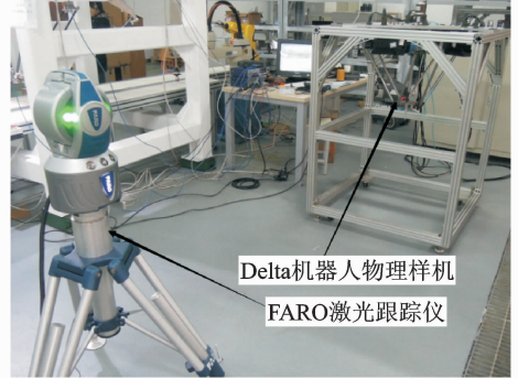
图 10 FARO 激光跟踪仪测量物理样机动平台运动轨迹 Fig.10 FARO laser tracker measuring moving platform trajectory of the physical prototype
