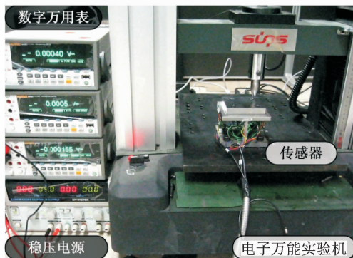
(b) 静态力测量实验环境 (b) Experimental setups for static force measurement
