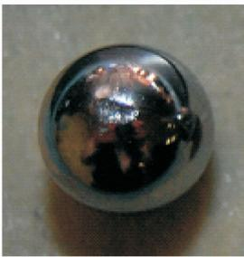
(c) 滚动体故障 (c) Rolling element fault
