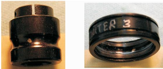
(a) 内圈故障 (a) Inner fault
