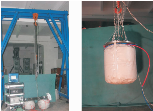
(a) 试验平台 (b) 竖直圆柱式气囊 (a) Experimental platform (b) Vertical cylindrical airbag
