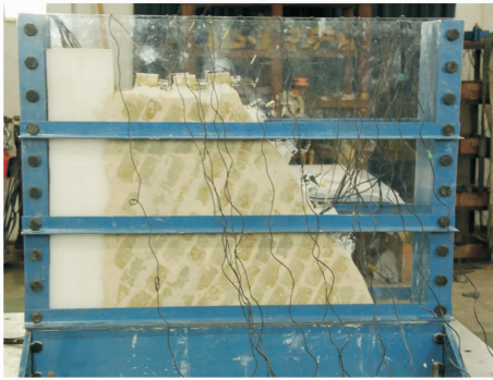
图 2 反倾岩质边坡模型的概化简图和完成的传感器布置图 Fig. 2 Schematic diagram and photographs of complete the sensors of anti-dip slope model
