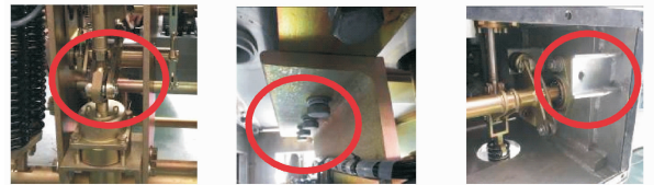
(a) 传动机构故障 (b) 基座螺丝松动 (c) 缓冲弹簧无效故障 (a) Actuator fault (b) Base screw loosened (c) Buffer spring invalid
