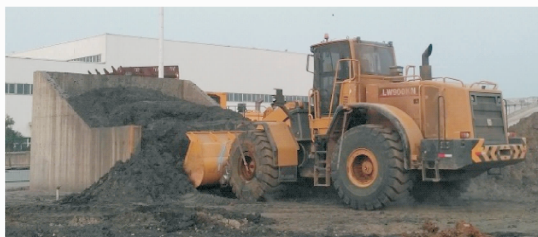
图8 铲装铁矿粉物料载荷测试试验 Fig. 8 Load test of iron ore material
