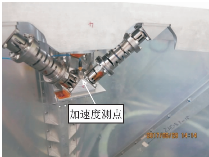
图 5 载荷隔振装置与星体连接位置处的加速度测点 Fig. 5 Acceleration measuring point at the position where payload isolator device is connected to the satellite
