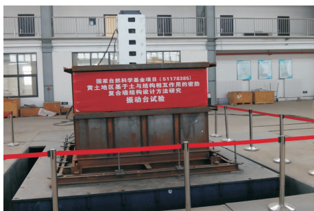
图 4 密肋复合墙结构与地基相互作用体系试验模型 Fig. 4 Model of interaction system of multi-ribbed wall structure and subsoil
