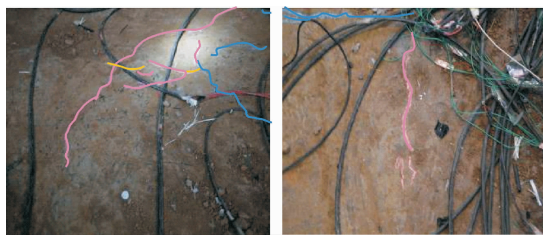
图 10 9 度后地基土表面裂缝 Fig. 10 Crack of subsoil surface under 9 degree
