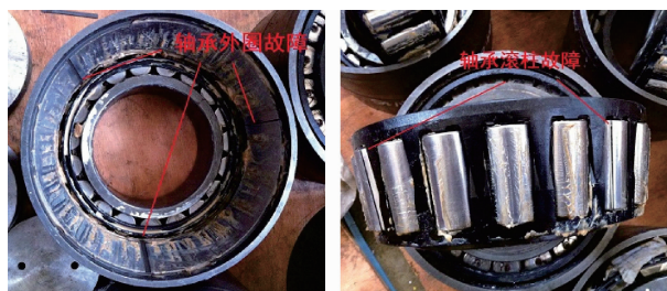
(a) 轴承外圈故障 (b) 轴承滚柱故障 (a) Outer ring fault of bearing (b) Bearing fault of bearing
