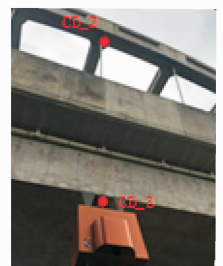
(c) 吊杆两端测点 (c) Measuring points at both ends of the boom
