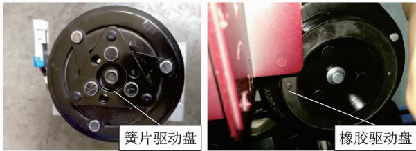
(a) 簧片驱动盘 (a) Reed drive plate (b) 橡胶驱动盘 (b) Rubber drive plate
