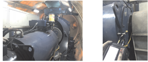
(a) 风力发电机传动链 (a) Wind turbine drive chain (b) 被测轴承 (b) The tested bearing
