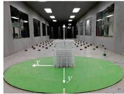
(b)  $0^\circ$ 风向角测压试验(b) HFPI wind tunnel test at  $0^\circ$  wind angle
