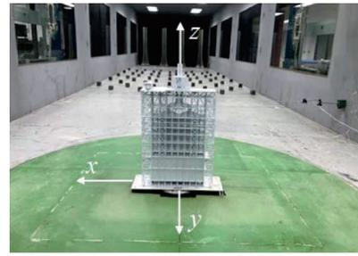
(a)  $0^\circ$ 风向角测力试验(a) HFFB wind tunnel test at  $0^\circ$  wind angle
