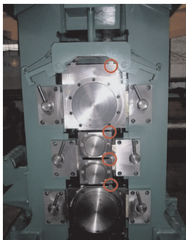
图3 四辊轧机垂直振动测试传感器现场安装位置 Fig.3 Installation position of sensor for vertical vibration testing of four-high rolling mill
