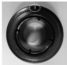
图 4 滚动轴承外圈故障 Fig.4 Rolling bearing outer ring failure
