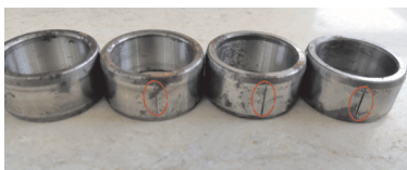
图 3 不同故障程度的轴承内圈 Fig.3 Bearing inner ring of different fault degree
