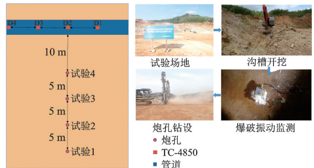
图6 爆破试验场地及炮孔布置 Fig.6 Blasting test site and hole layout
