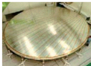
(c) 12 m 充气天线结构 (c) Inflatable antenna structure with a diameter of 12 m
