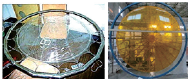
(a) 1 m 充气天线结构 (a) Inflatable antenna structure with a diameter of 1 m (b) 3 m 充气天线结构 (b) Inflatable antenna structure with a diameter of 3 m
