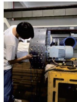
图3 频响函数测试 Fig.3 Frequency response test
