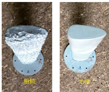
图2 粗糙的导线雾凇覆冰模型与光滑的导线雨凇覆冰模型 Fig.2 Rough model of rime icing conductor and smooth model of glaze icing conductor
