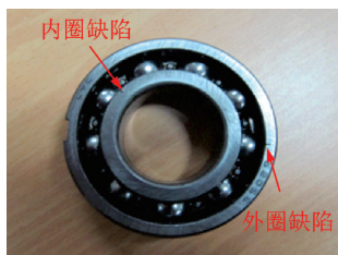
图 5 轴承的故障位置 Fig.5 Failure site of bearing
