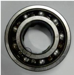
(b) Failure bearing of inner ring
