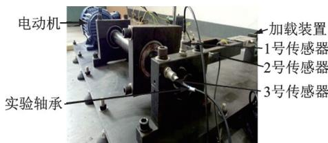
(a) Rolling bearing simulation failure test bench
