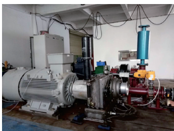
图5 高速离心压缩机整机综合性能试验台 Fig.5 Performance test bench for high-speed centrifugal compressor
