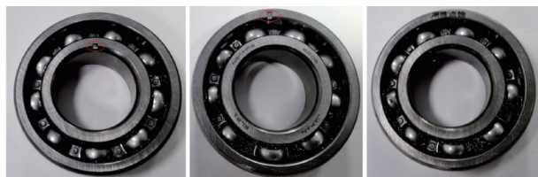
(a) 内圈故障 (a) Inner ring fault (b) 外圈故障 (b) Outer ring fault (c) 滚动体故障 (c) Rolling element fault
