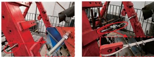
(a) 螺栓连接 (a) Bolted connection (b) 卡扣连接 (b) Buckle connection
