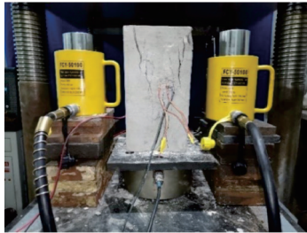
(b) 试块表面破坏情况 (b) Surface damage of test block
