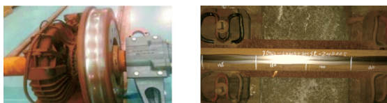
(a) 车轮多边形 (a) Wheel polygon (b) 钢轨波磨 (b) Rail corrugation
