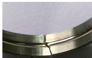
图 11 CSF-14-80 型柔性薄壁轴承及外圈故障断裂状态 Fig.11 CSF-14-80 flexible thin-walled bearing and fracture state of outer ring
