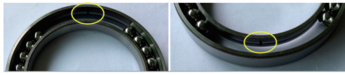
(a) 外圈缺陷 (a) Outer ring defect (b) 内圈缺陷 (b) Inner ring defect
