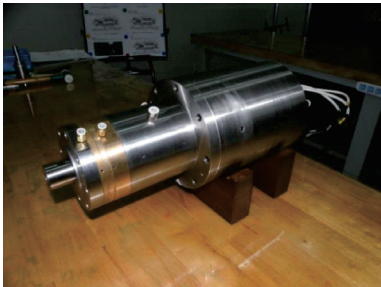
图 13 高速水润滑动压螺旋槽轴承电主轴试验样机 Fig.13 The test prototype of the motorized spindle with water-lubricated hydrodynamic spiral groove bearing
