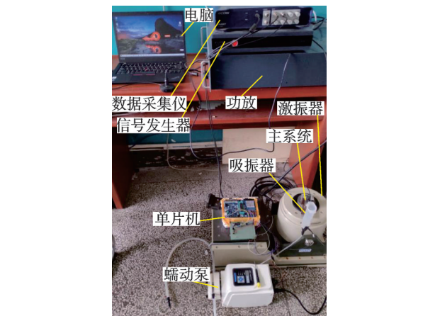
图10 实验系统 Fig.10 Photograph of the experimental system
