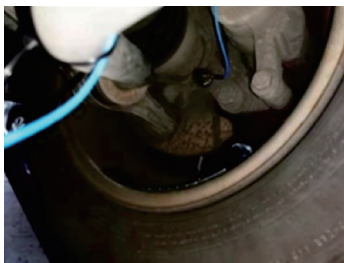
图3 传感器位置 Fig.3 Acceleration sensor location
