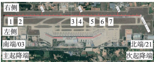
图 11 横坡坡度过大处沿跑道分布图 Fig.11 Steeply transverse slope distribution along the runway
