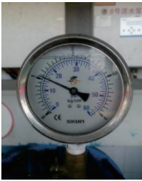
图6 关机过程中最大压力对应压力表(单位:Pa) Fig.6 Maximum pressure corresponding to pressure gauge during shutdown (unit: Pa)
