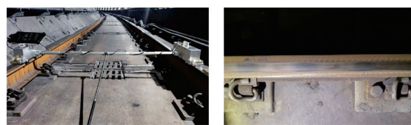
(a) 钢轨波磨仪 (b) 钢轨波磨 (a) Rail corrugation measuring instrument (b) Rail corrugation
