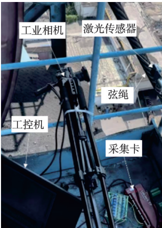
图6 煤矿现场实验系统 Fig.6 Experiment system at coal mine field
