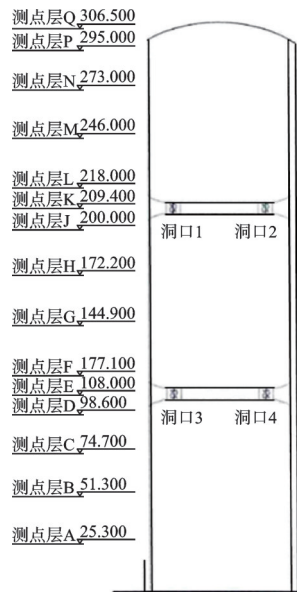
图3 风洞试验测压点布置(单位:m) Fig.3 Layout of measuring points for wind tunnel tests (unit: mm)
