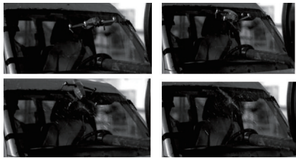
图 10 无人机以 15 m/s 速度撞击贴膜汽车前风挡玻璃试验过程 Fig.10 Test process of UAV impacting coated car front windshield at 15 m/s
