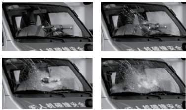
图 13 无人机以 40 m/s 速度撞击贴膜汽车前风挡玻璃试验过程 Fig.13 Test process of UAV impacting coated car front windshield at 40 m/s
