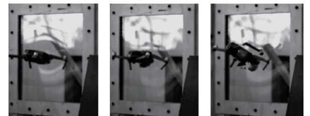
图 15 无人机以 30 m/s 速度撞击高铁侧风挡玻璃试验过程 Fig.15 Test process of UAV impacting high-speed train side windshield at 30 m/s
