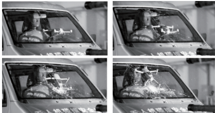
图 11 无人机以 25 m/s 速度撞击贴膜汽车前风挡玻璃试验过程 Fig.11 Test process of UAV impacting coated car front windshield at 25 m/s
